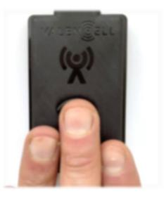
Fig. 1: Valencell developed and validated a novel machine learning model, based on PPG datasets collected from thousands of unique participants, to estimate BP via finger PPG.
